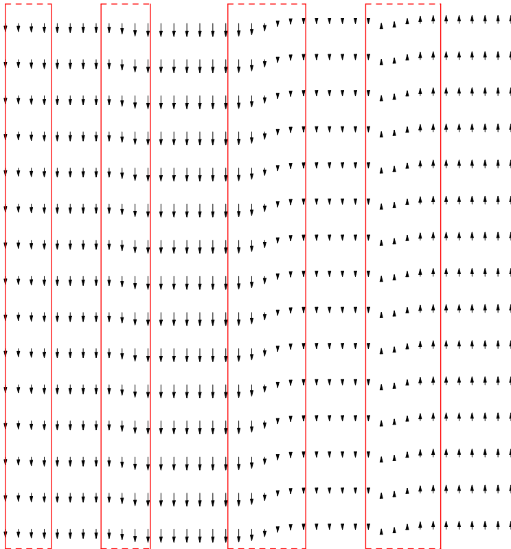
Fig 18. The 2D magnetic field corresponding to the current sheets in fig. 17. The solid and dotted red lines indicate the current sheet structures.
