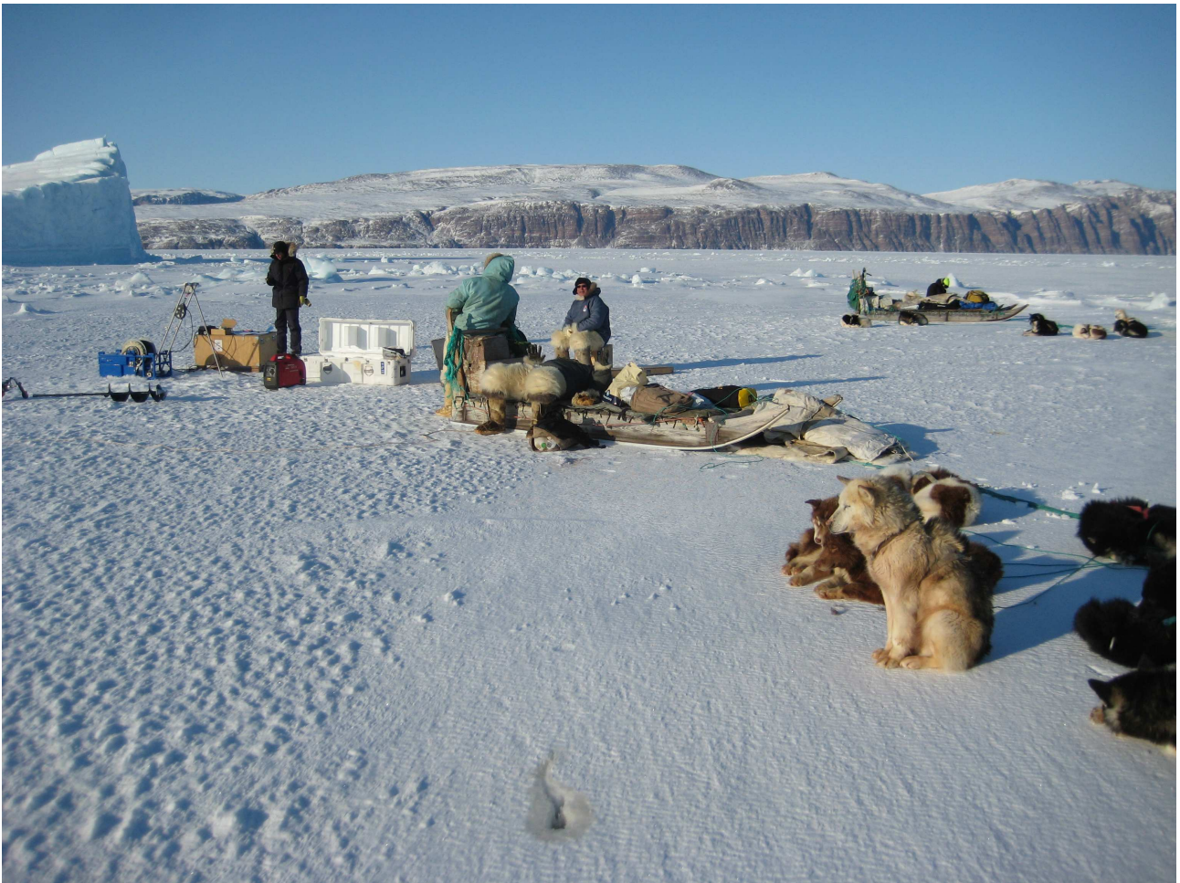
Figure 13 Oceanographic measurements in the bottom of Inglefield Bredning. The CTD is lowered into the water from the tripod on the left and the EM-31 is hidden on the sledge in the background.
