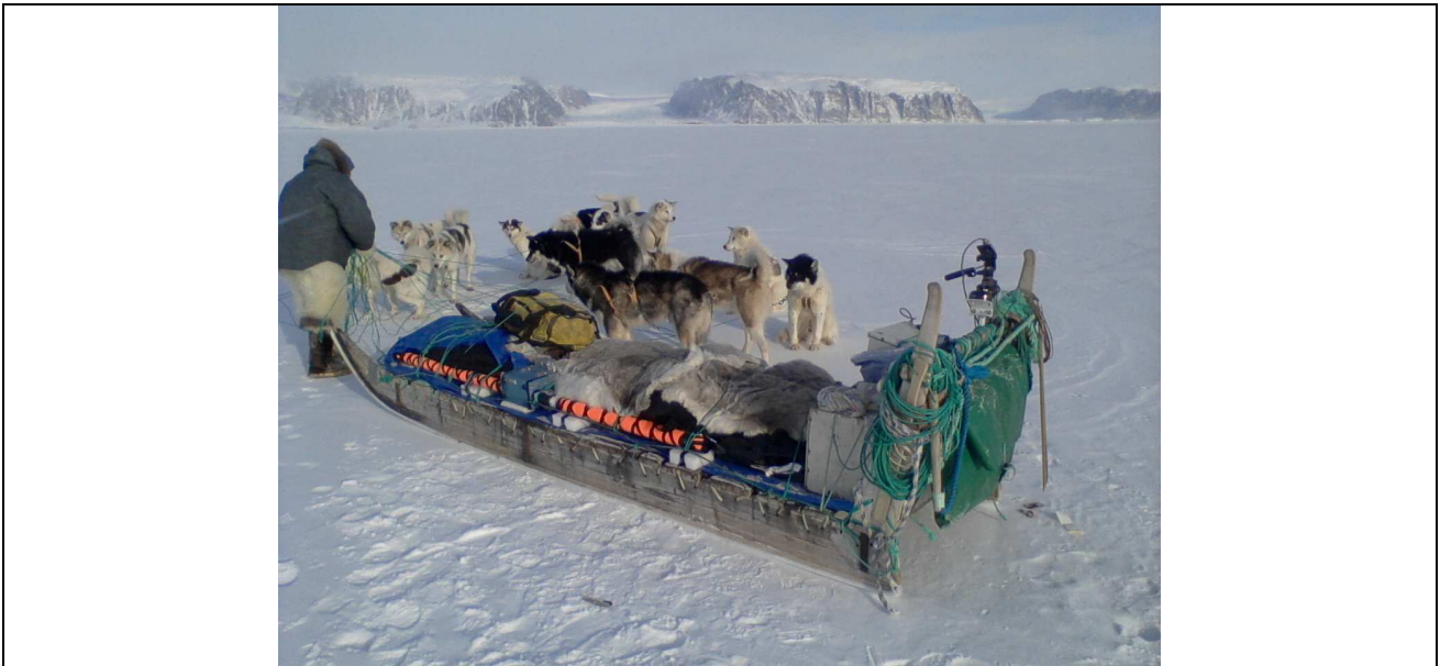
Figure 9 Em-31 wrapped up on a dog sledge and ready to go. The IR100 radiometer is seen by the right handle at the back of the sledge.
