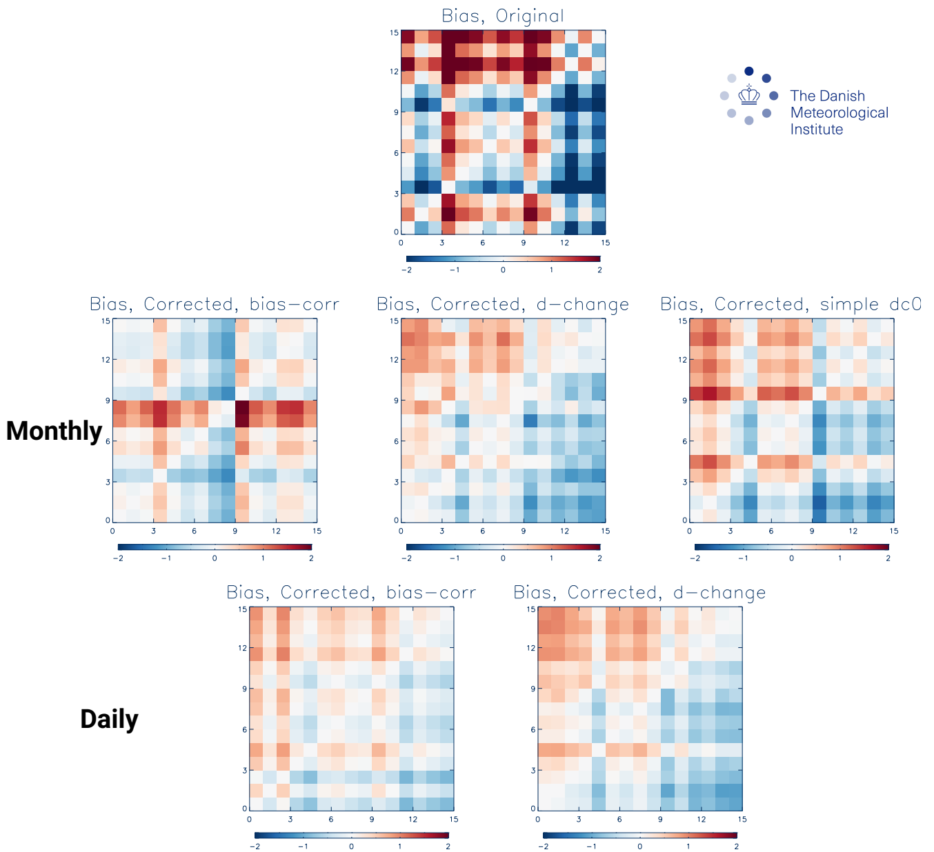
Figure 7: The difference between mean climates in calibrated models and ‘truth’. January near-surface temperature. Calibration period 1971-2000, prediction period: 2070-2099. Scenario: RCP8.5. The numbers on the axes refer to the model combinations in Table 2. The horizontal axes indicates the model selected as ‘truth’. Top panel shows uncalibrated values. In middle panes calibration is performed on monthly means, in lower panels on daily means.
