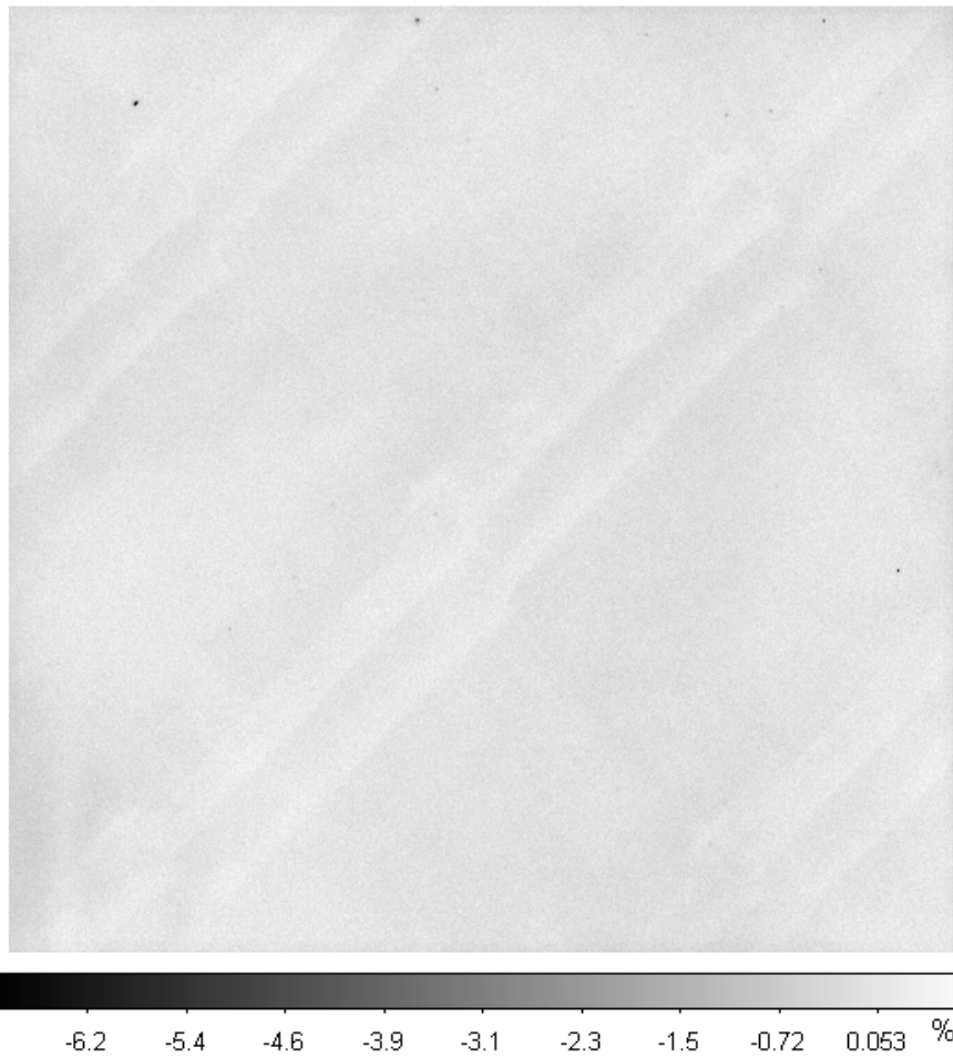
Figure C.9: Percent difference image in the IRCUT-filter between twilight master flatfields from JD 2455827 and JD 2455831. Some of the bad pixels close to the edge of the frame can still be seen.
