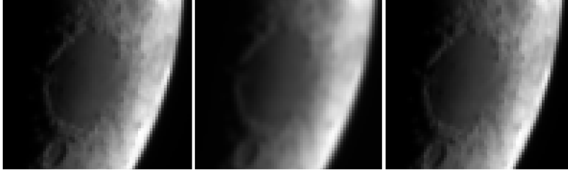
Figure 7.1: Alignment of a single Moon image from session JD 2455864. Zoom on the Crisium crater. Left: Raw image before alignment. Middle: After alignment with center-of-mass method. There is visible blurring of lunar features. Right: After alignment with Chae's method. There is no visible blurring of lunar features.
