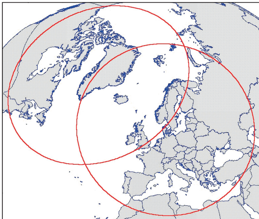
Figure 9. Coverage of DMI's NOAA ground stations in Denmark and Greenland.
