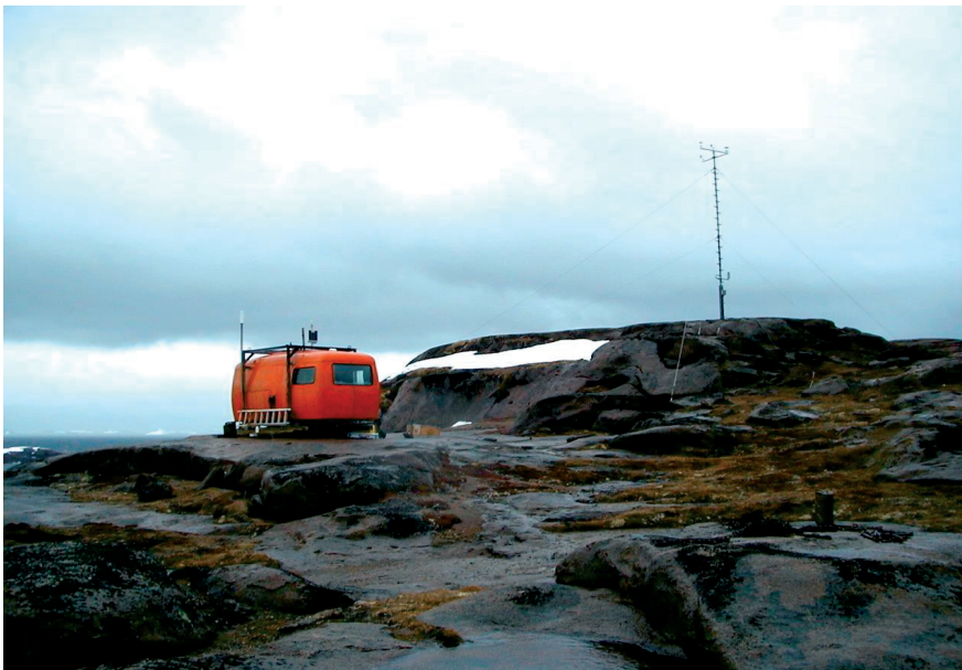
Figure 4. Remote station in Nunarssuit, Greenland. Operating automatic weather stations at remote sites in the high arctics represents a considerable technical and logistic challenge. The stations are solar powered, and during the short summer they need to collect enough energy for the four months of arctic winter night with temperatures below -40^{\circ}\text{C} . The most northern stations are serviced only once every second year. The remote stations send their data to DMI's satellite receiving stations in Kangerlussuaq, Greenland and Copenhagen via the ARGOS system.
