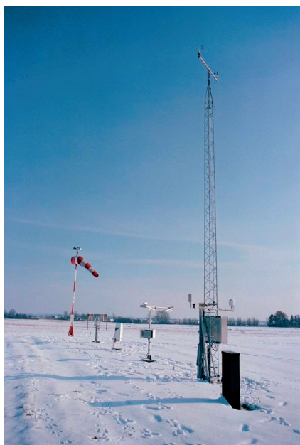
Figure 3. Automatic V98 weather station at Holbaek Airport, Zealand, Denmark. The station is fully equipped with optical sensors for present weather and cloud parameters.
